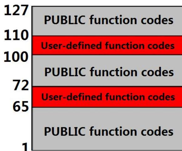
Figure 51 Modbus Function Codes
