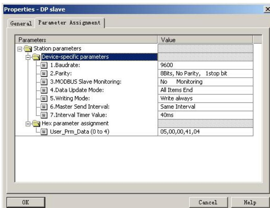
Figure 14 G0306-MS Configuration of Device User Parameter
