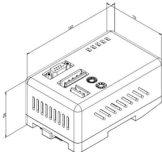
Figure 2 Gateway Outline Dimensional Drawing (112\*70\*50, unit mm)
