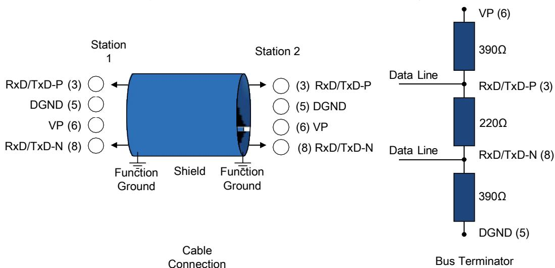
Figure 8 RS485 Transmission Technology Wiring and Bus Terminator
