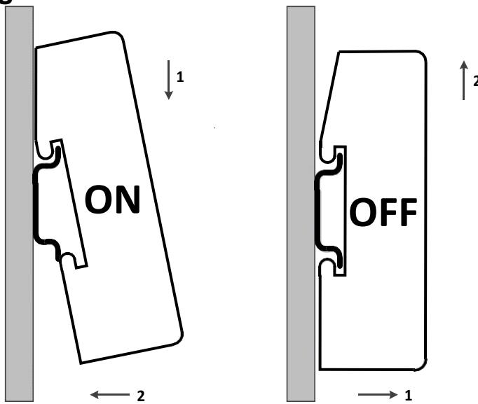
Figure 4 DIN Guide Rail Installation
