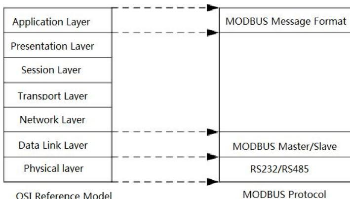
Figure 50 Modbus Protocol Model
